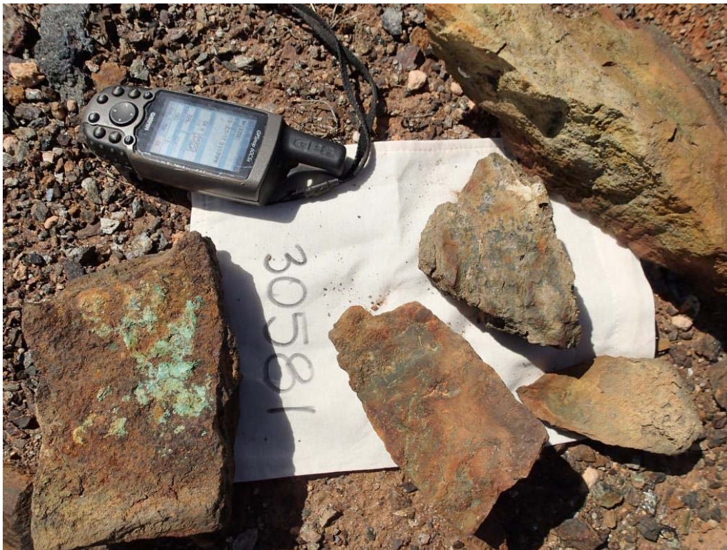
Plate 1 Gossanous and copper-bearing magnetite-rich sample (no. 30581) to northeast of Copper Blow.
