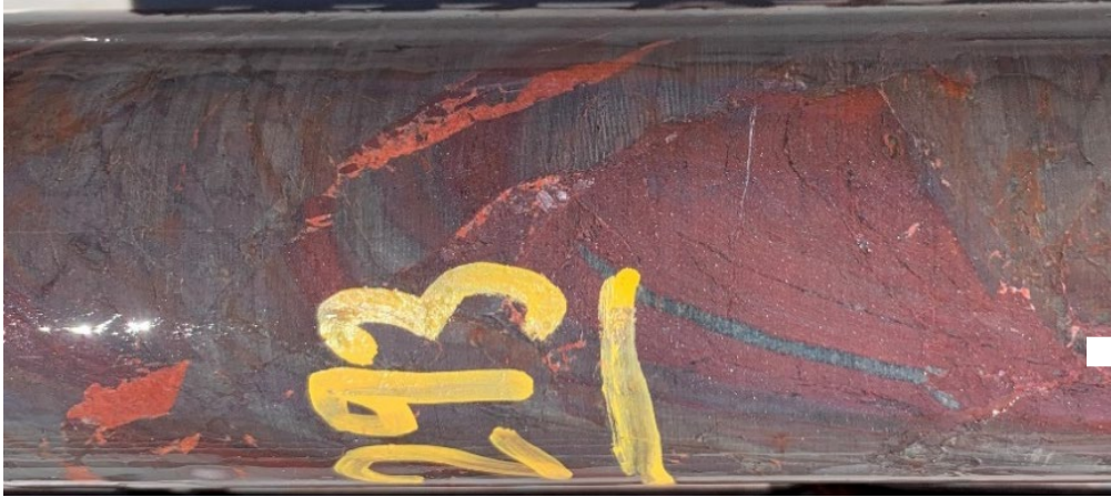
Figure 4: Faulted hematitic shale with later cross-cutting K-feldspar in-fill. Hole depth: 293m.
