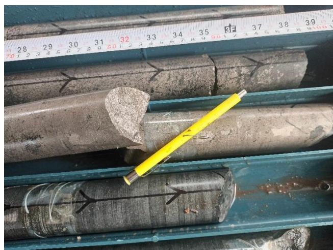
Figure 3: Massive sulphide unit from 423.4m to 423.6m DDLUHC005
