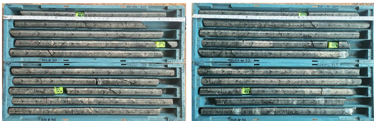
Figure 1 and 2: Zone of semi-massive and heavily disseminated nickel sulphide mineralisation 408m and 423m in DDLUHC005
