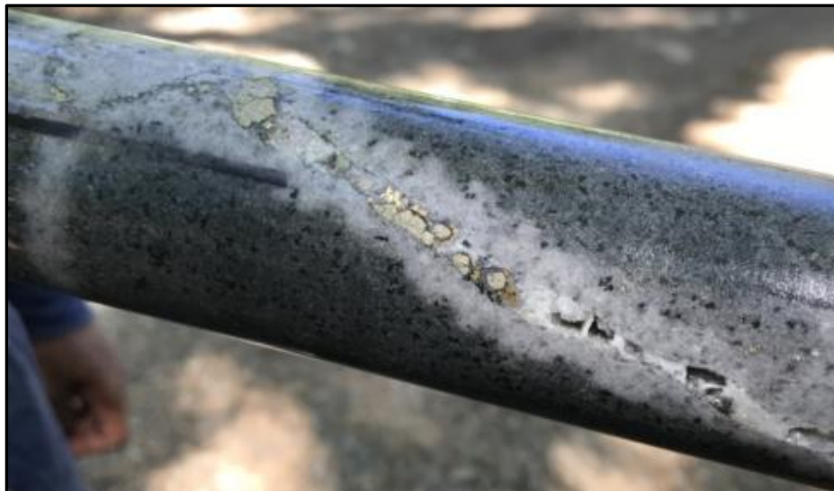
Photo: drill core from mineralized interval in diamond drill hole TUDDH-500
