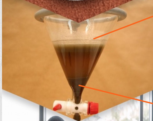
Photo 5. Laboratory HM separation via a heavy liquid
