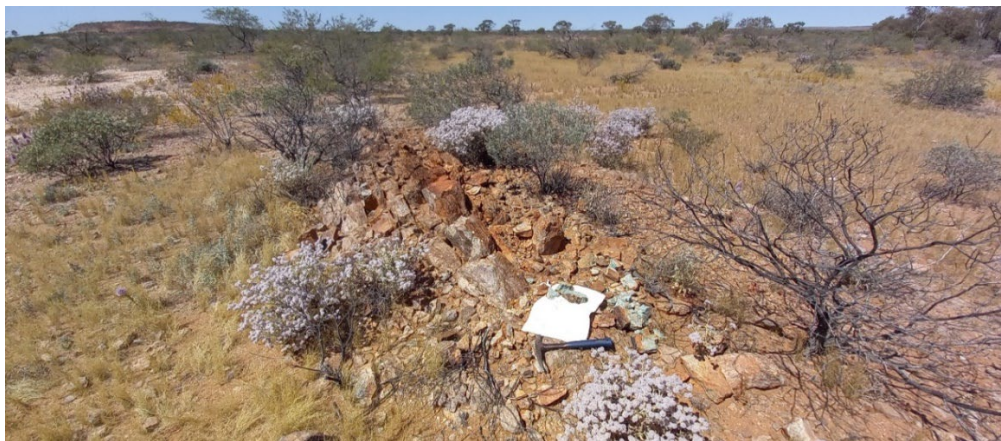
Figure 9: VMS base-metal target; exhalative malachite, chalcocite, and galena-bearing barite lens.
