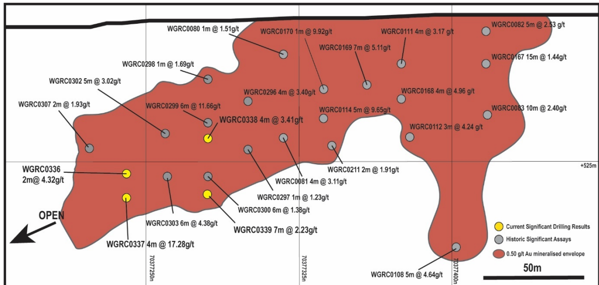
Figure 3 – Eastern BIF south long section (facing west). Recent drill results with yellow markers, historic drilling in grey. Mineralisation remains open at depth and to south. Section width 80m
