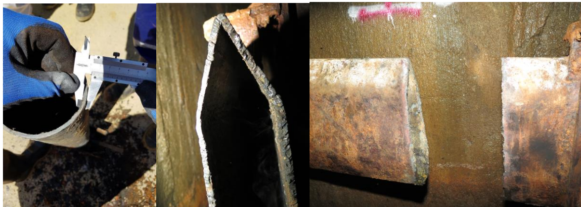
Figure 8: (LHS) Divider from submerged Bunton Set number 81 tested steel thickness to 5.0mm; (Middle) section through retrieved Bunton (RHS) location where bunton section was removed.
