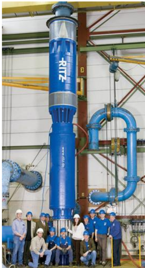
Figure 9: A Ritz pump recently used for mine dewatering at an operation in the Democratic Republic of Congo.
