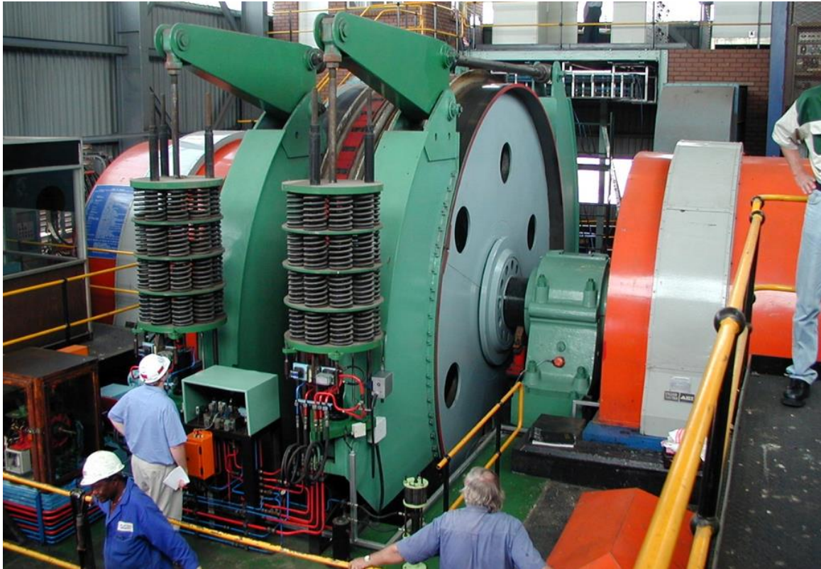
Figure 6: The original Hutchings Shaft rock winder in use currently at a South African mining operation.
