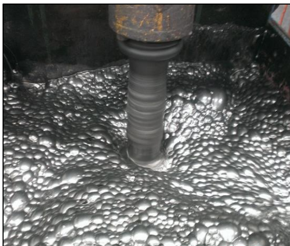
Figure 1. Flotation cell concentrating flake graphite
