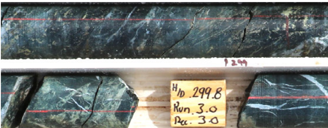
Figure 2 - AWT003 drill core at 299.0m: chalcopyrite (copper) and pyrite zone in a strongly silicified sheet vein (leakage structure) contained within strong propylitic altered volcanoclastic greywacke and basalt sequence.
