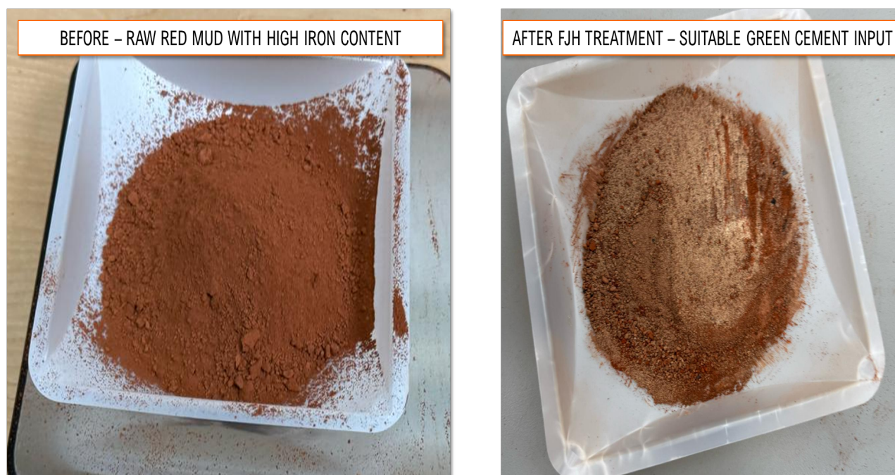
Figure 5: Photo of high iron content Red Mud feedstock and resultant low iron & low sodium product
