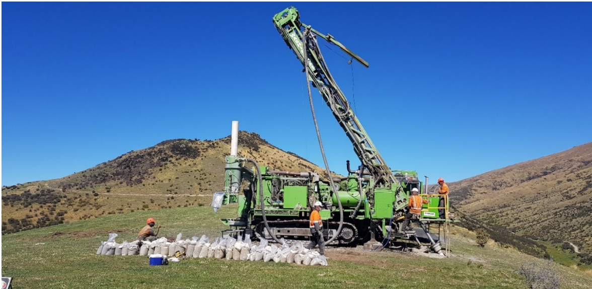
Figure 5: RAS RC drilling (MRC079)
