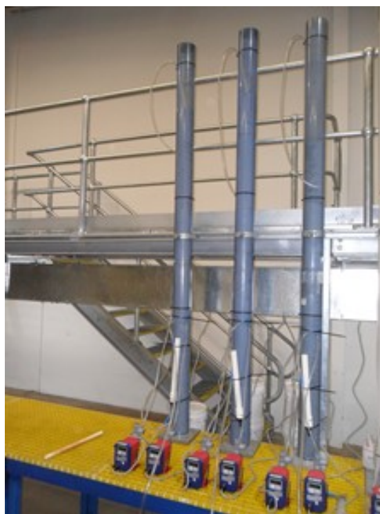
Figure 17: Column leach tests on CIT, RAS and SRE sulphide ore
