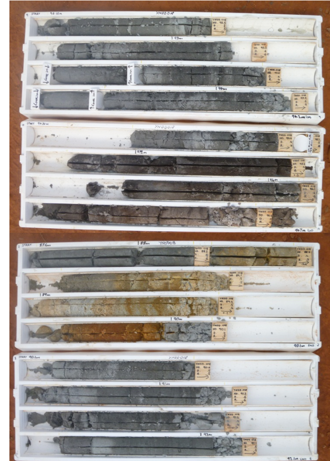
Core from Yanrey Project's Bennet Well South: trays show the sedimentary contrasts and are coincident with the gamma spikes
