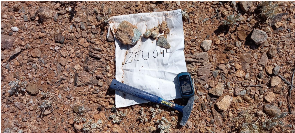
Figure 6. Sub-cropping exhalative malachite, chalcocite and galena bearing barite lens, (Sample# ZEU044 = 2.19% Cu, 0.2% Pb)
