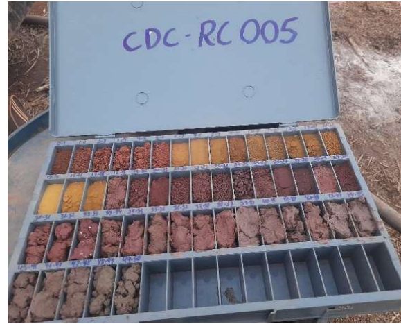
Figure 9: Variegated colour of drill cuttings from CDC-RC-0005 hole, implying changes in lithology across undifferentiated sediment, laterite, kamafugite
