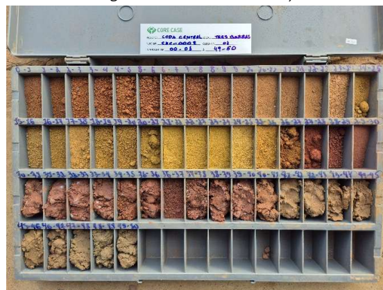
Figure 4: Cuttings from CDC-RC-0002 drillhole showing reddish brown to off yellow Kamafugite
