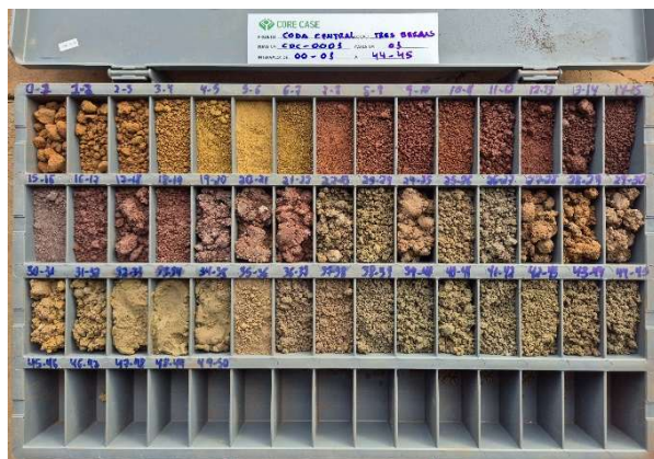
Figure 3: Cuttings from CDC-RC-0001 drillhole showing reddish brown Kamafugite and hole ended in mineralisation
