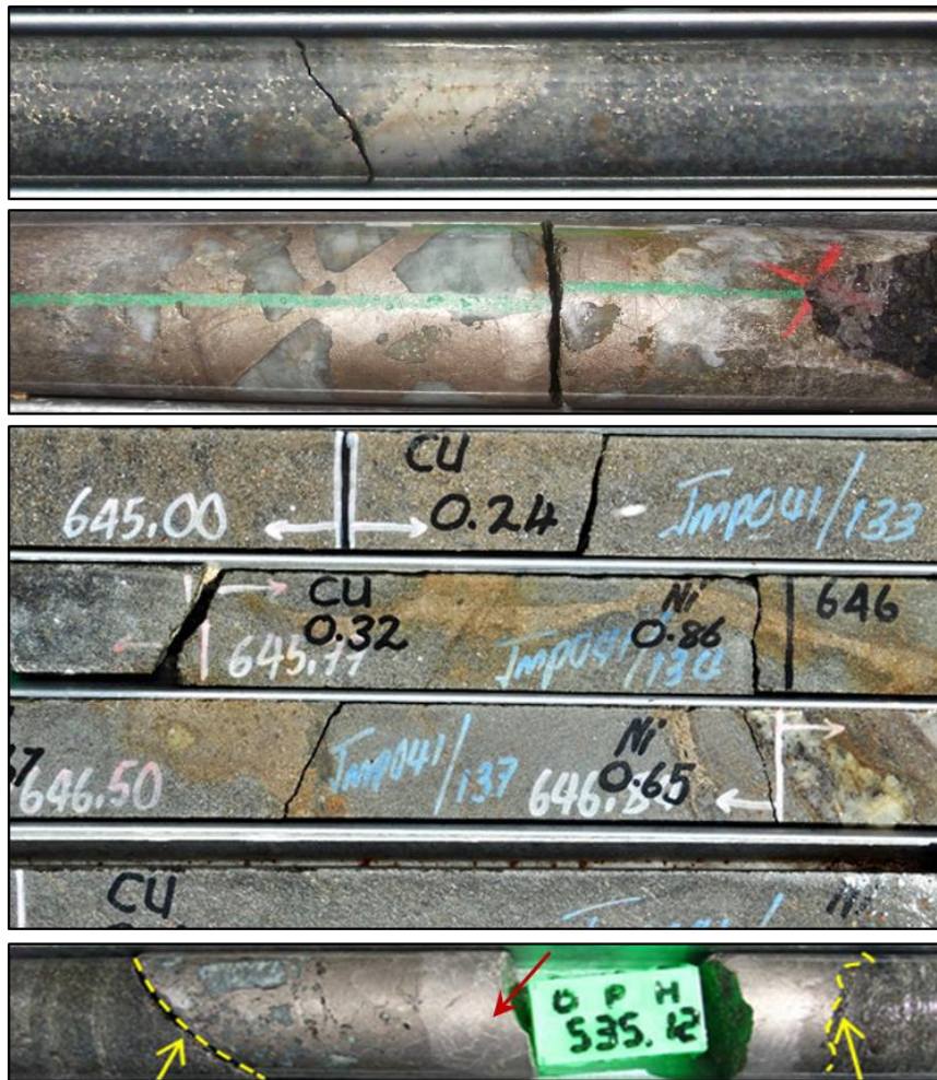
Figure 14: Type 2 mineralisation hosted by all lithological units at Jacomynspan. From the top; massive sulphide stringer (JMP001) with an associated alteration halo cross-cutting the peridotite unit. Massive sulphide vein associated with pegmatitic feldspar (JMP003) cross-cutting the pyroxenite unit. Transgressive massive sulphide veins intruding and brecciating already-lithified pyroxenite unit (JMP041). Massive sulphide stringer, which is currently unique due to its higher tenor (>4% Ni), and which has coarse loop texture (red arrow) (JMP038).
