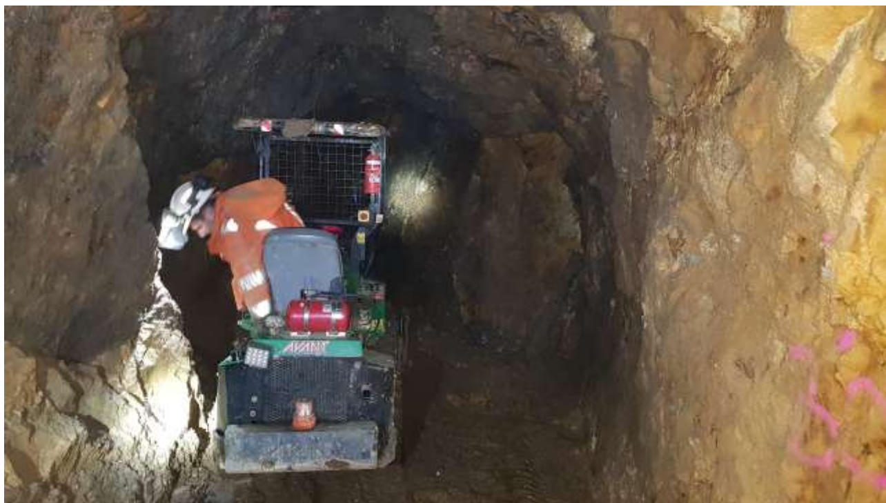
Figure 2 - Ore being loaded from the face of the Mystery Drive
