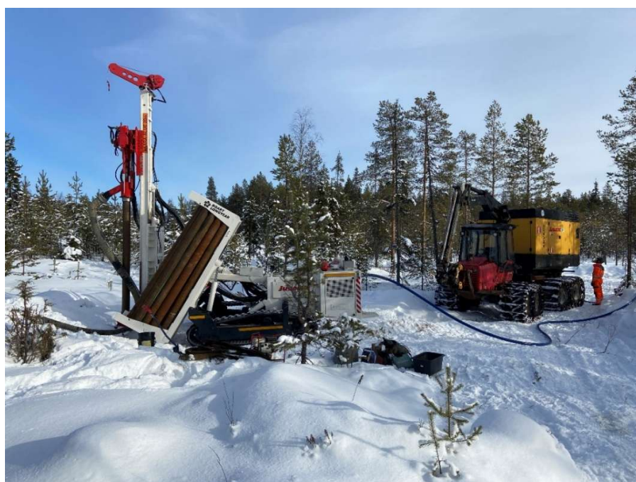
Figure 9: RC drilling at K6E
