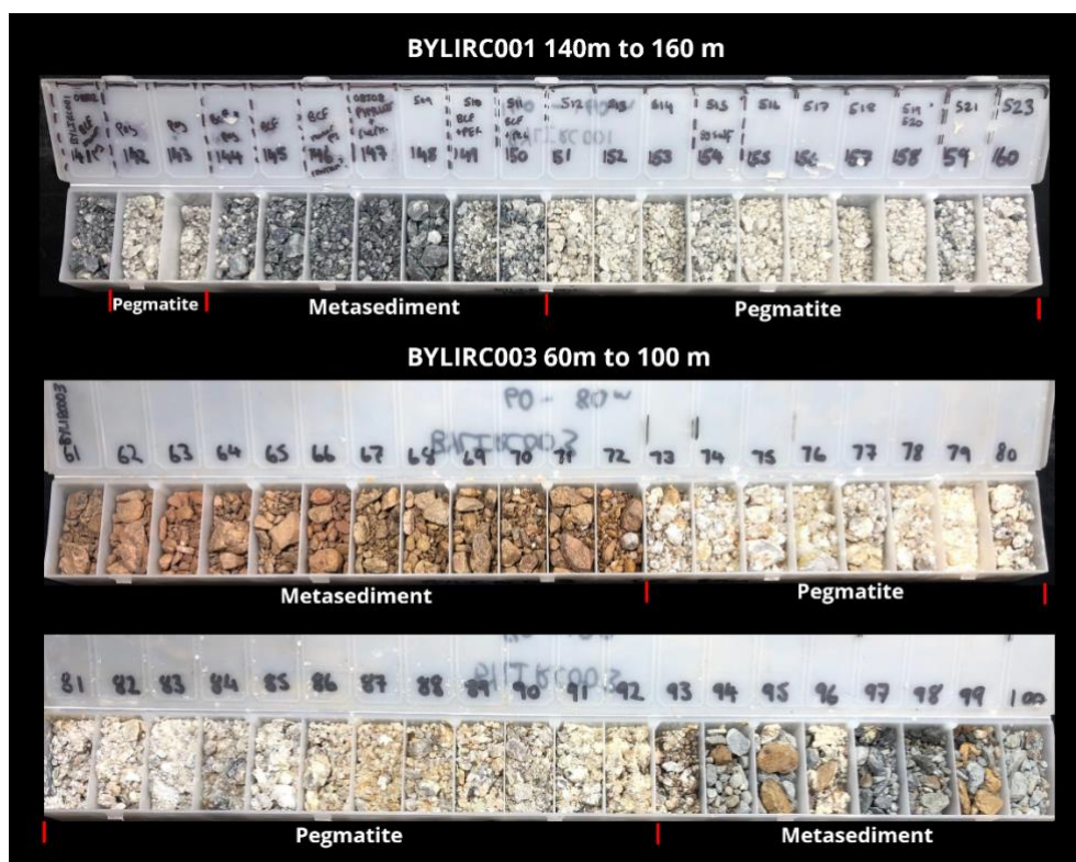
Figure 2: Selected RC chip sample trays for BYLIRC001 and BYLIRC003.
