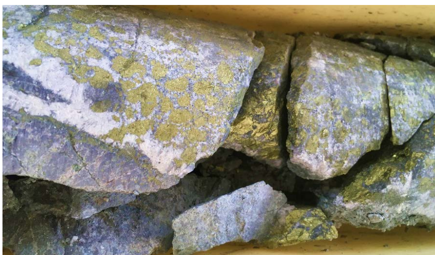
Figure 1. Chalcopryite-carbonate vein in rhyolite porphyry, BWDD076 (70.1m) which assayed 5% copper over 1m.
