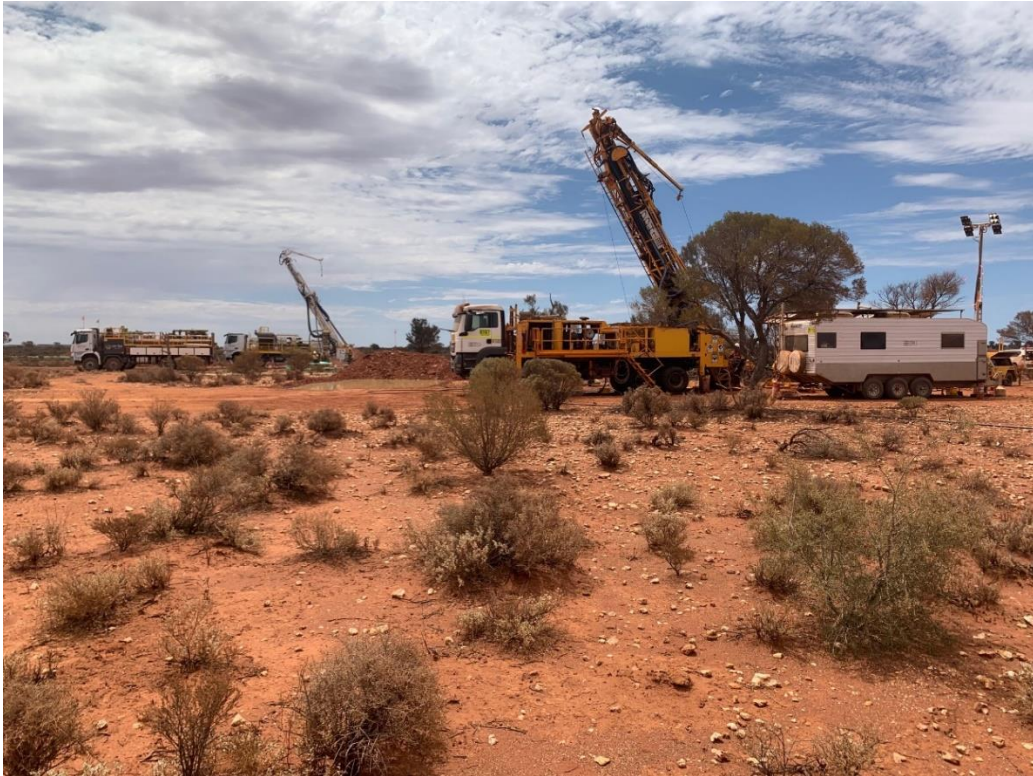
Photo 1: Crusader – Templar Prospect RC and diamond drill rigs in operation
