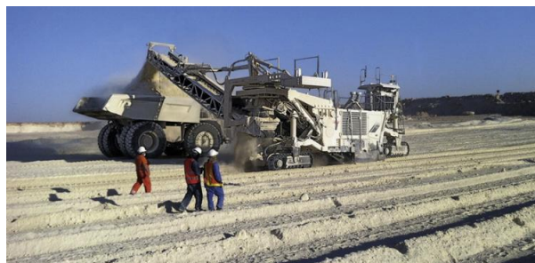
Fig 1 - Example Surface Miner – Limestone row cutting
