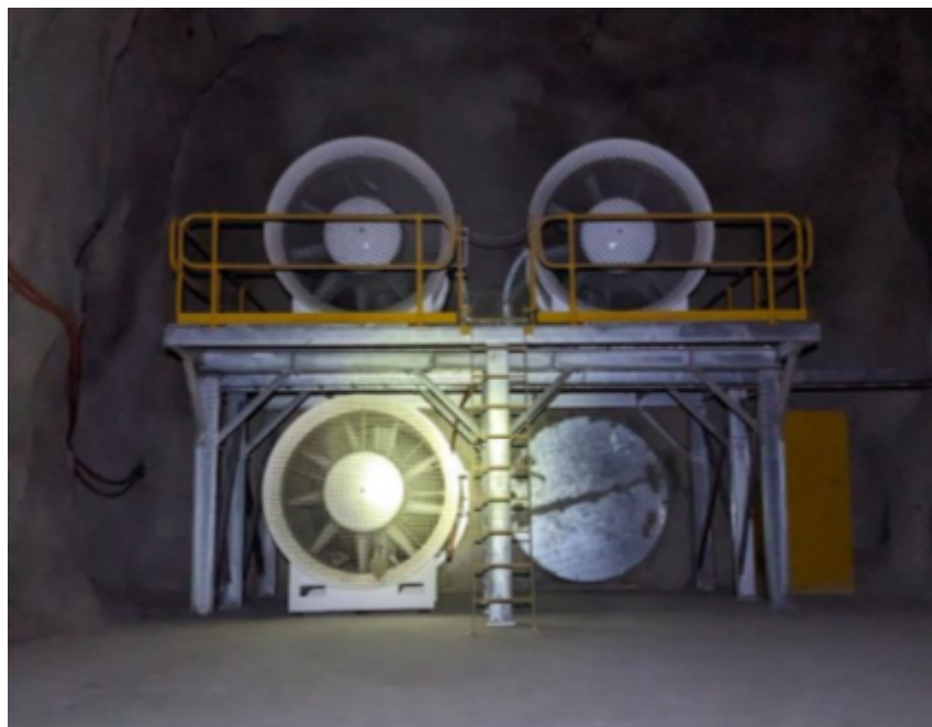
Figure 7 Indicative sub-terrain ventilation setup proposed for Sand King, image from Riverina Gold Mine
