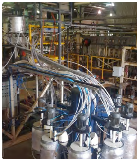
Resin-in-Pulp circuit at SGS Metallurgy pilot plant
