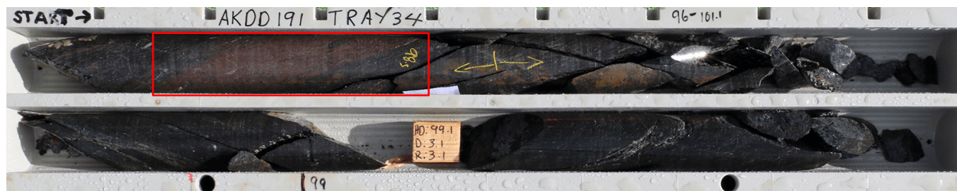
AKDD191 core samples including intersection of massive sphalerite and minor galena from 97.8 m to 98.5 m
