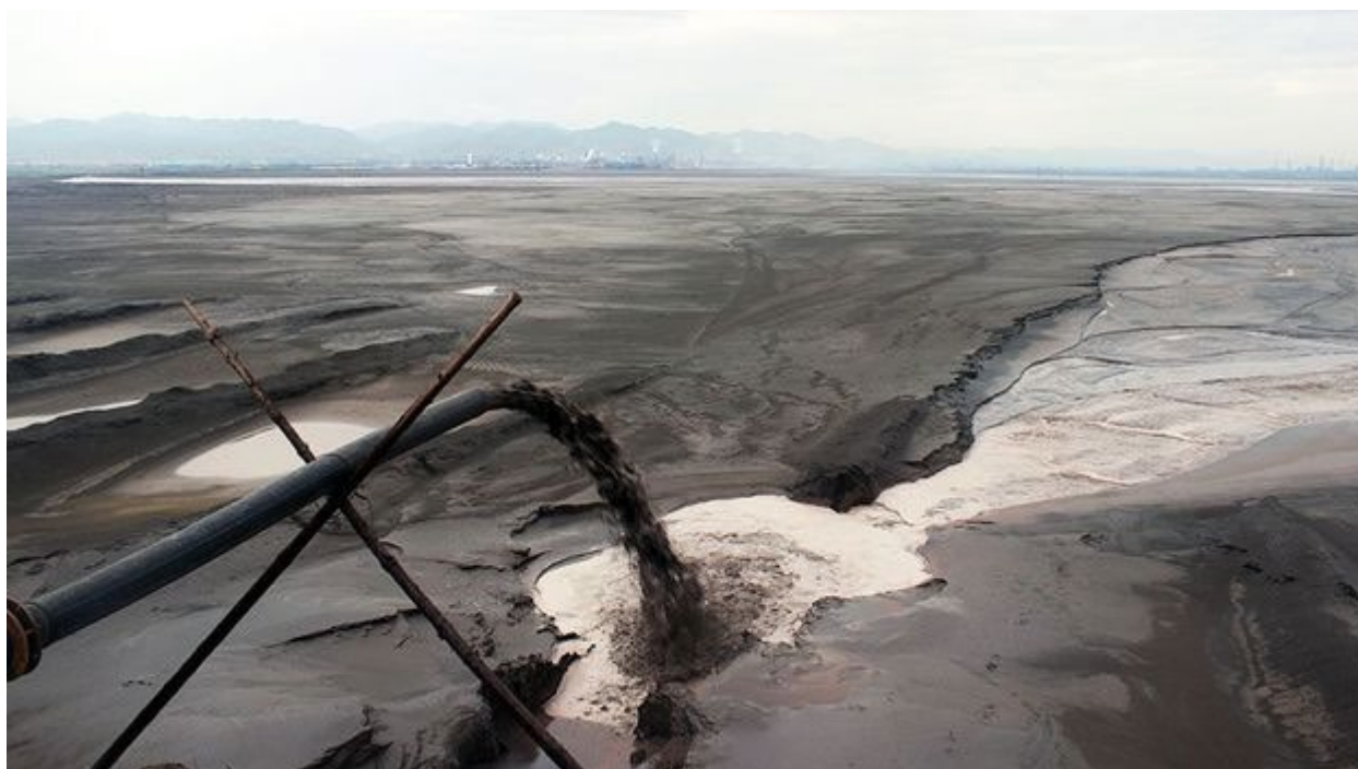
Figure 1: Tailings generated from conventional rare earth production, Inner Mongolia, PRC.
