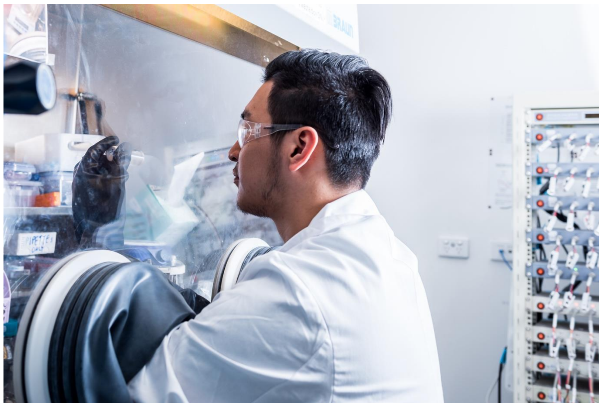
Image 1. Battery materials formulation, assembly and testing incorporating Archer Campoona graphite being performed at UNSW.
