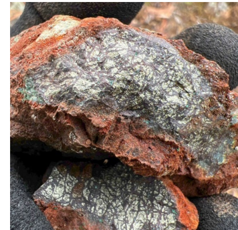
Back Barb – malachite in sheared ultramafic outcrop; 10cm wide vein with secondary chalcocite and relic primary chalcopyrite 1
