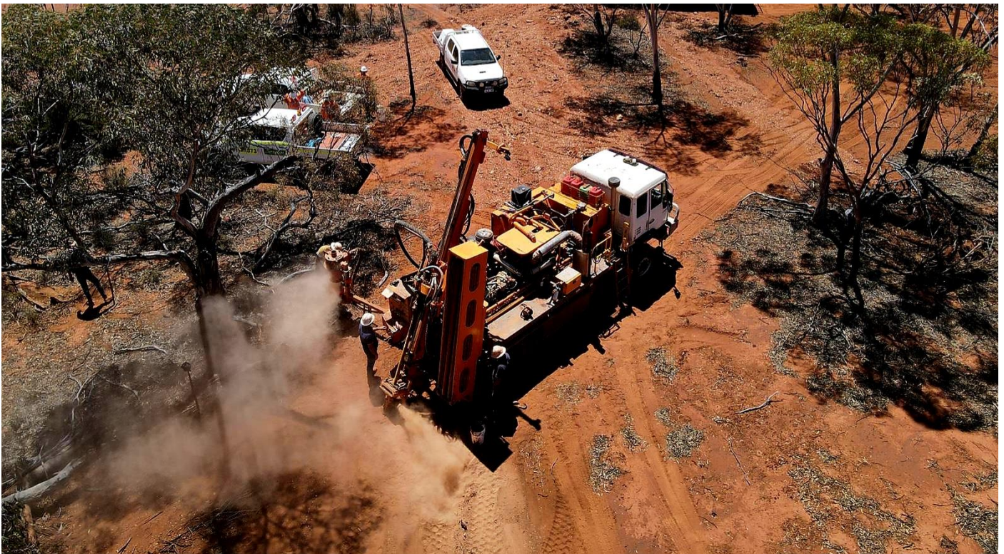
Figure 1 - KTE Mining Services air-core drill rig commencing drill programme at the Kemble gold prospect.
