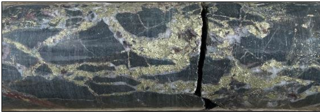
Photo 1. Chalcopyrite-quartz-hematite fill jigsaw breccia in chlorite-silica altered microdiorite - SMD173, 390.6m drill depth, HQ diameter uncut drill core. Note the dominance of chalcopyrite and hematite and the almost total lack of pyrite.
