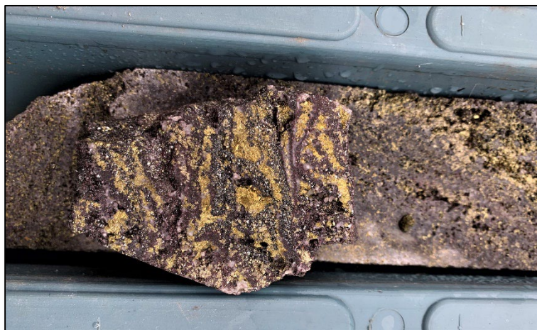
Photo 2. Chalcopyrite-specularite-hematite-magnetite mineralisation – SMD182, 423.5m drill depth, HQ3 diameter ½ cut drill core.
