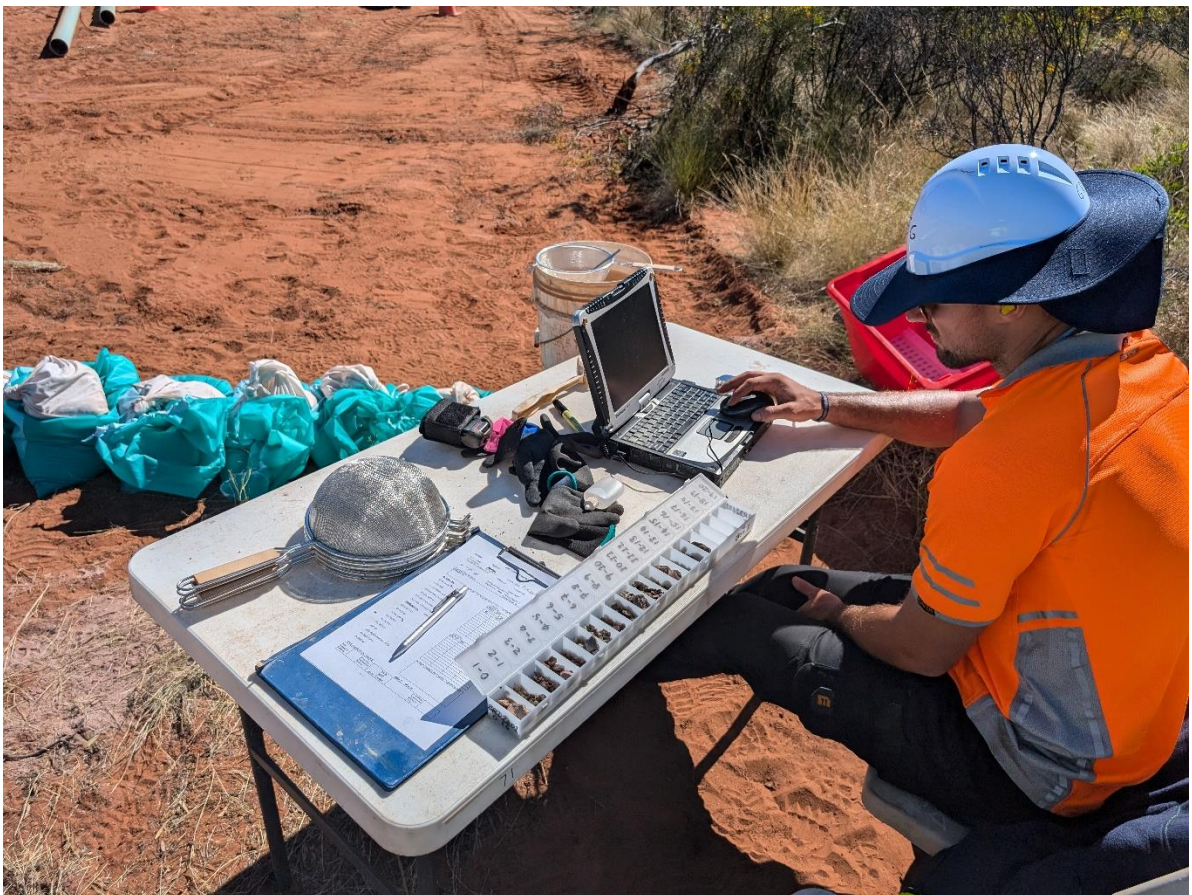
Figure 2: A geologist assesses and records every metre of the RC Drillhole
