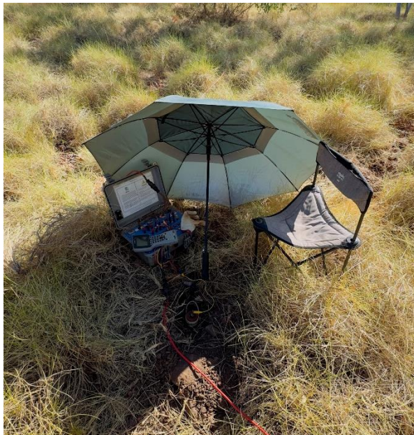
Figure 1 – Photographs from the recent IP survey at Paperbark, showing the equipment setup at a station (left) and laying out the cable in typical vegetation in the project area (right)
