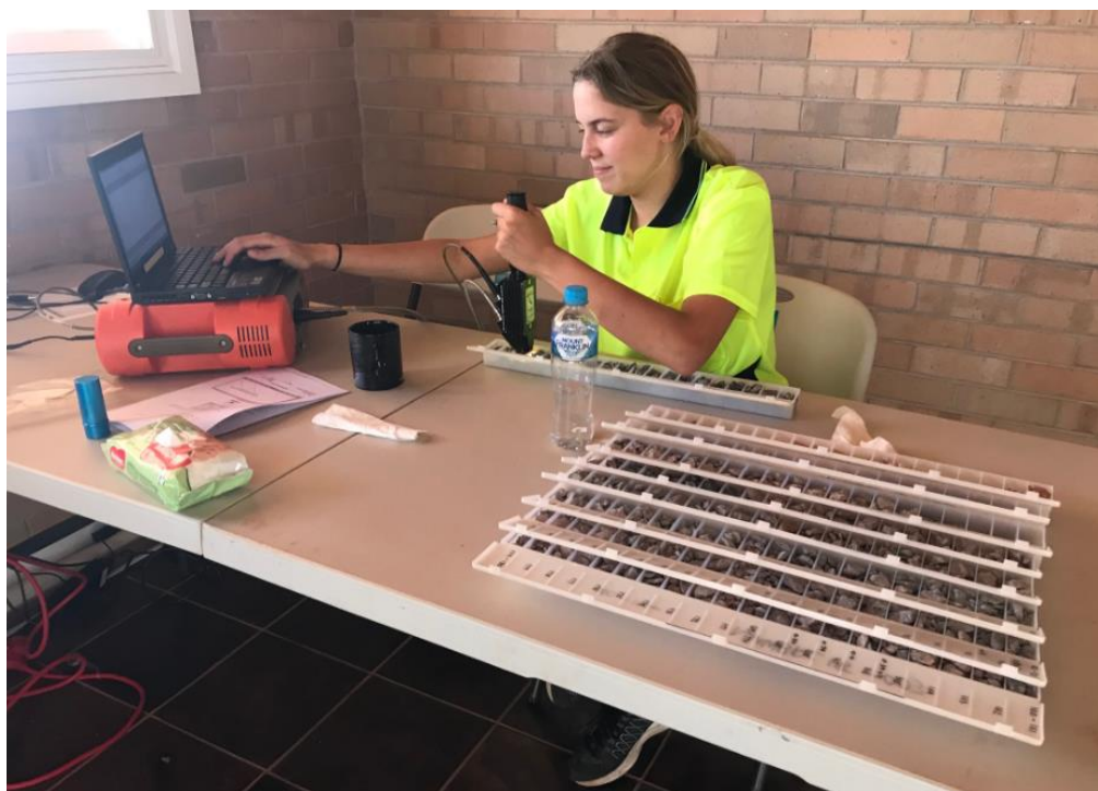
Photo 1: SWIR RC Drill Chip Sample Data Collection
