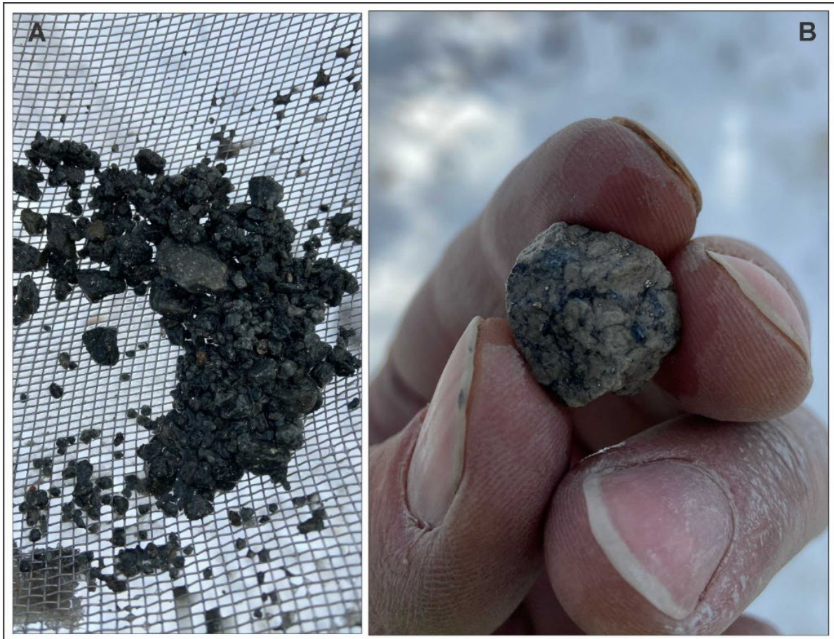
Figure 3: Visual sulphides intersected within K6RC009. A: Interval 4-5m, B: interval 14-15m
