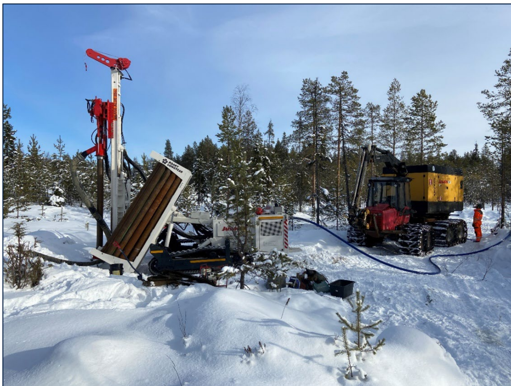
Figure 1: RC drilling at K6E
