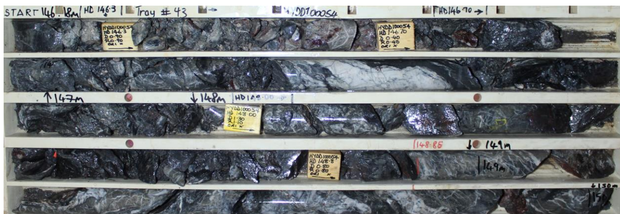
Figure 2 - Veining, sulphides, and alteration in diamond hole HYDD100054 similar to that seen in the 2018 RC drilling
