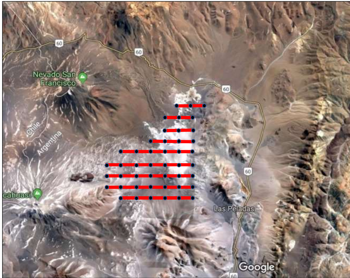
FIGURE – SAN FRANCISCO SALAR DRILLING PLAN. EXPLORATION PROGRAM WILL COMMENCE IN ARGENTINE SPRING 2019. IT INCLUDES SURFACE AUGERING AND ASSAYS, GEOPHYSICS AND DRILLING.
