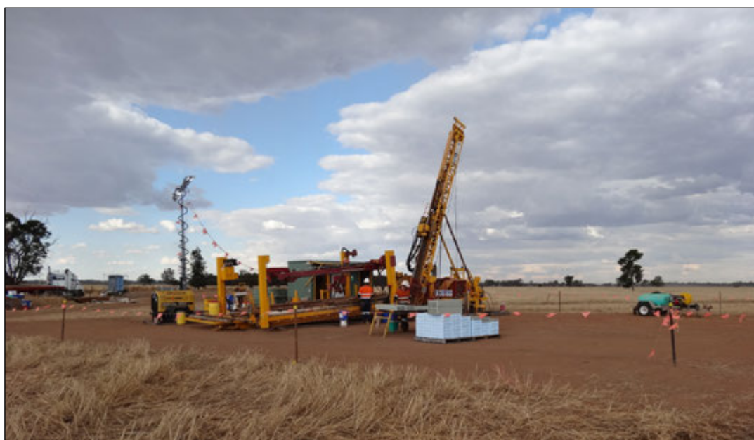
Figure 3 - Titeline Drilling Rig 8 – UDR200D drilling hole AWT001
