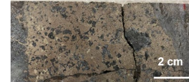
Massive sulphide in 20WGDD0005 (340.4 – 340.5m) grading 1.38% Ni
