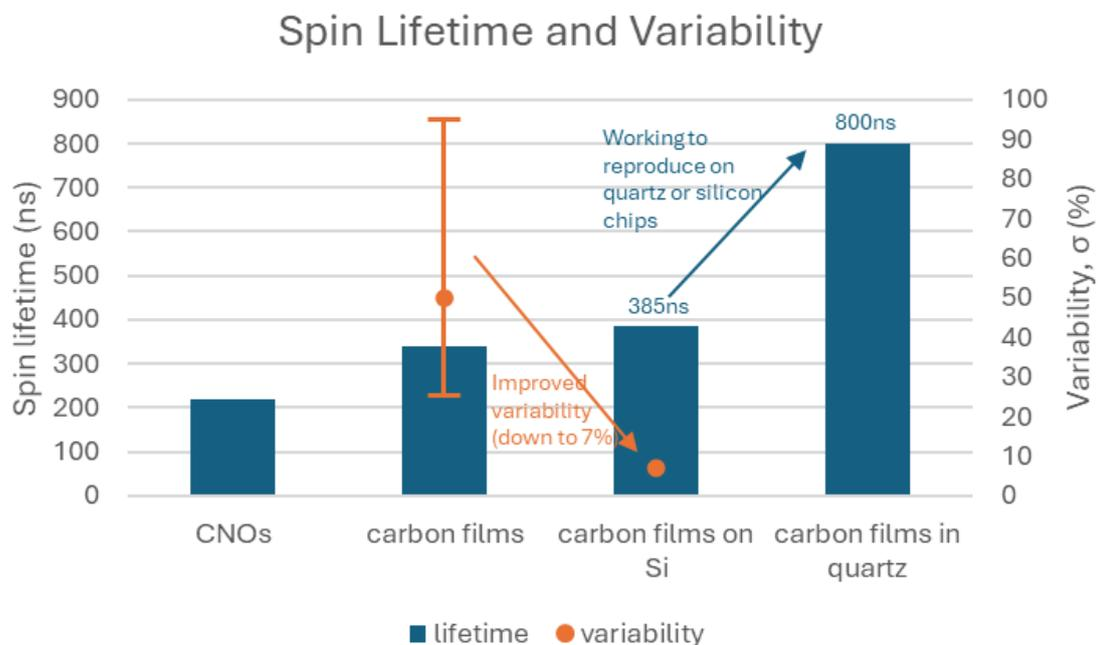
**Image 1.** Electron spin-lifetime has been increased to 800 ns under certain conditions. Work is in progress to repeat this to increase from 385 to 800 ns on chips. Significant improvements have been made on uniformity. Variability has been driven down from >25% to ~7%.
