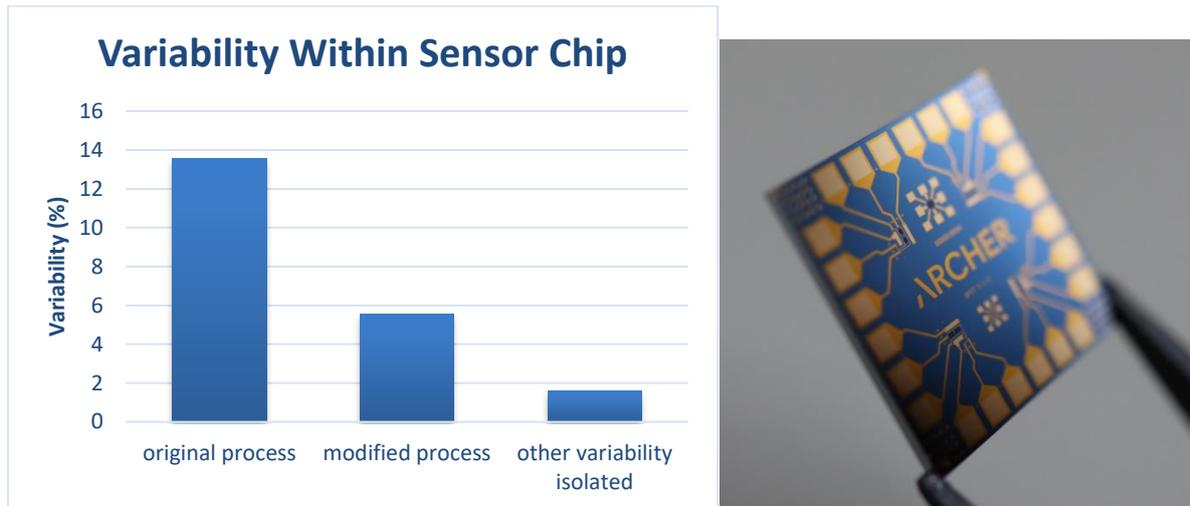
**Image 2.** The chart shows the variability of response to mM/l concentrations of potassium of gFET devices on a chip. The photograph shows Archer's sensor test chip. These chips contain several gFETs (barely visible). The liquid (currently mock samples, but later blood) is transferred to the chip in micro-litre volumes and the individual gFET responses are read.
