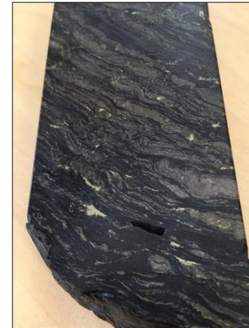
Disseminated chalcopyrite in carbonaceous shale
