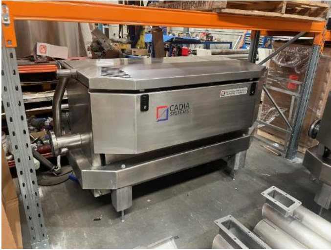
NMR's new Cadia electrowinning cells and extraction system
