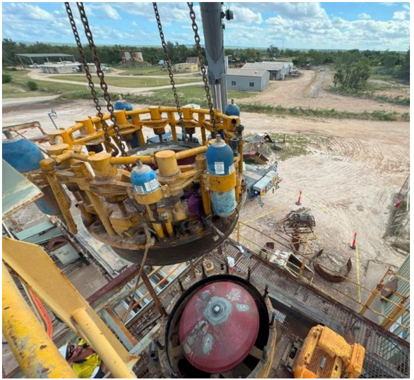
Area 01 - Final refurbishment of cone crusher
