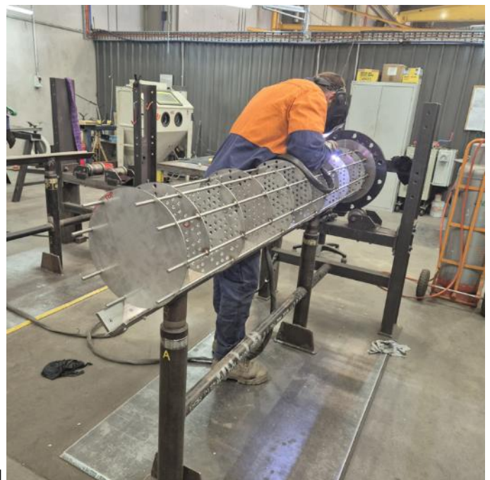
NMR's new elution heater from Gasco - vessel body & bundle cage
