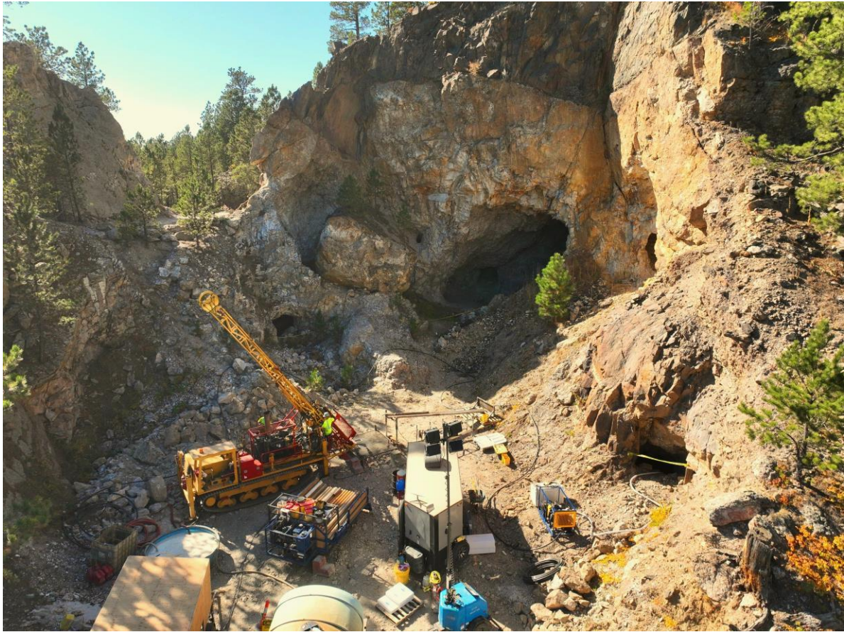
Figure 3: Active core drilling operations at the Tin Mountain Project.
