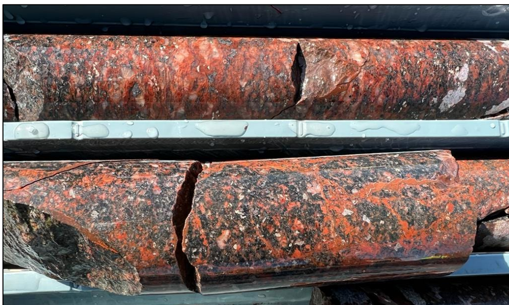
Figure 3. Pervasive iron oxide staining together with magnetite and sericite alteration of the host granite (HELIOS_DD002)
