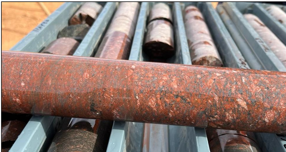
Figure 2. Pervasive iron oxide staining and hematite in altered granitic host rocks (HELIOS_DD002)
