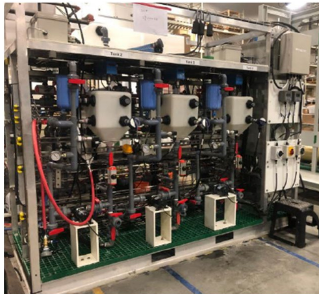
Figure 3: Pilot Scale Lithium Carbonate and Wash Equipment
