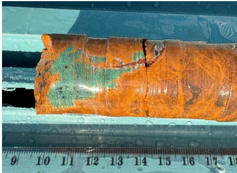
Figure 5: Copper (malachite) in oxidised dolomite/ankerite host vein of WYPC08 at Worrumba 22.
