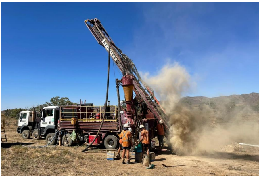
Figure 1: First RC hole WCRC001 being collared at the Wyacca Prospect.
