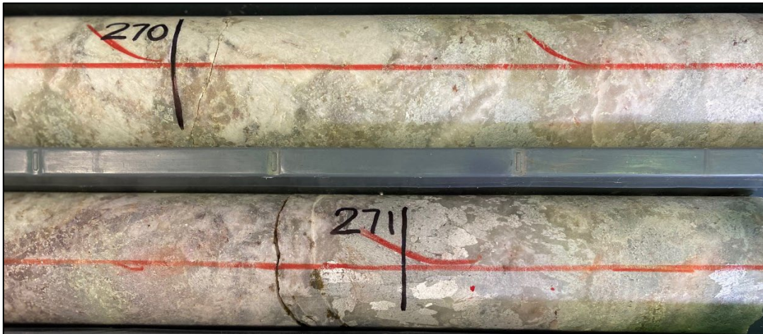
Figure 2: Boxed core sample from BYLDD003 between 270m and 271m downhole.
