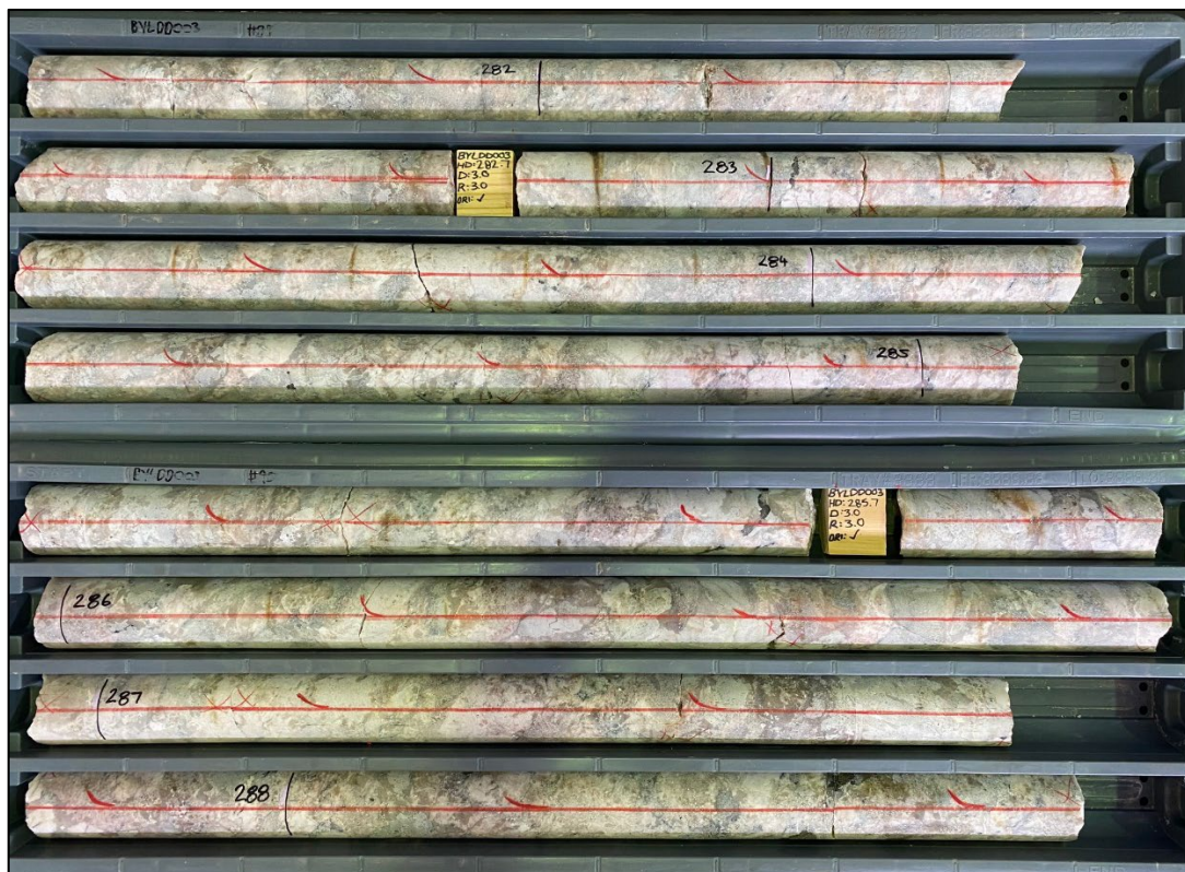
Figure 1: Boxed core sample from BYLDD003 between 281m and 289m downhole.
