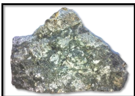
Figure 11a) Brecciated Dacitic Porphyry with disseminated chalcopyrite and chalcocite from the base of the Carmelita workings (~50m below surface) on the eastern edge of Target 1. Sample assayed 3.1% Cu, 0.1g/t Au, 11g/t Ag and 200ppm Mo 1 .
