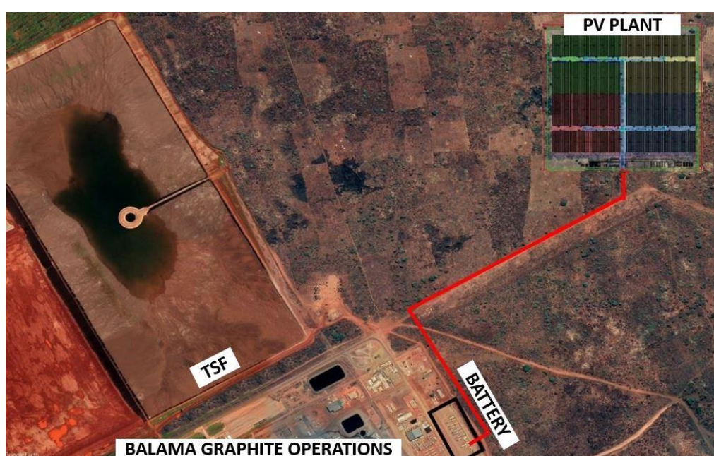
Figure 1: Schematic layout of solar and battery installation.
