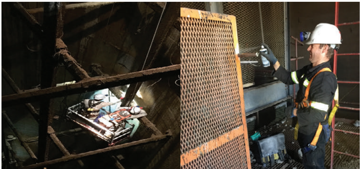
Figure 10: (LHS) Visual Inspection of Hutchings Shaft (RHS) Non-destructive testing of Hutching Headframe
